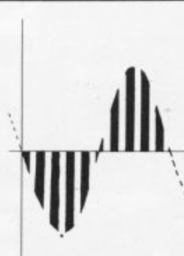
Fig. 2a] The sine wave chopped [sampled] by a 10 kHz pulsed signal.
