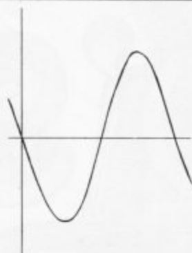
Fig. 1a] A full cycle of a sine wave at 1 kHz.
